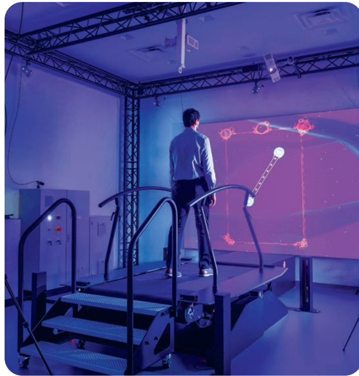
^ The Gait Real-time Interactive Laboratory (GRAIL) is projecting the subject's foot placement on the screen.
